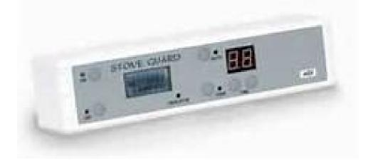
This device is a motion detector and can tell if there is movement within twelve feet of your cooktop. Figure the amount of time you are usually away from the stove during a normal meal prep and set the detector for more than that time. Then when the Stove Guard doesn't note motion for more than the span of time, the stove is shut off.
