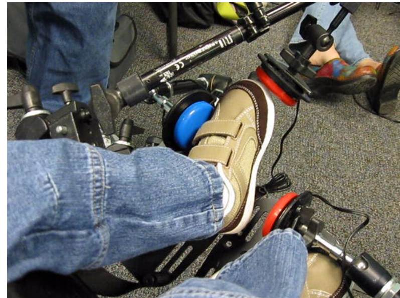
AbleNet Jellybean switches and Universal Switch Mounting Systems (UMS)
