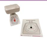
INSTRUCTOR: Show construction of the face of the scale on the Student Tool: Dial Scale Model by locating the numerals for pounds and lines for ounces. Remove the cover of the scale and locate on the actual scale as well. Count the amount of ounces in a pound (16) and 1/2 pound (8). Show there is only one line for every two ounces on the actual scale.
